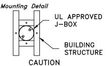
HARDWARE PACKET "A" MOUNTS DIRECTLY TO BUILDING STRUCTURE.
