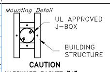
HARDWARE PACKET "A" MOUNTS DIRECTLY TO BUILDING STRUCTURE.
